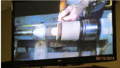
17. Remove the steps with a parting tool or gouge. The underside of a spindle gouge can help you make smooth cuts. Use any tool you are comfortable with that fits in the space.
