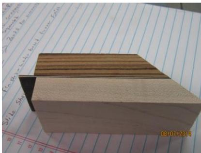
2. Once the glue has dried you can cut these in pieces at a 45 degree angle. A 1/8 backer on the chop saw will help get a cleaner cut.
